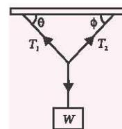
17. A mass of 5 kg is suspended in equilibrium, by two light inextensible strings  $S_1$  and  $S_2$  which make angle of  $30^\circ$  and  $45^\circ$  respectively with the horizontal. Then (Take  $g = 10 \text{ m s}^{-2}$ )
